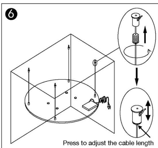
Thread the suspension wire through the hole in the ceiling mount pieces. Screw in the threaded locking pieces finger-tight. Do not fully tighten. Repeat for all 4 pieces.
