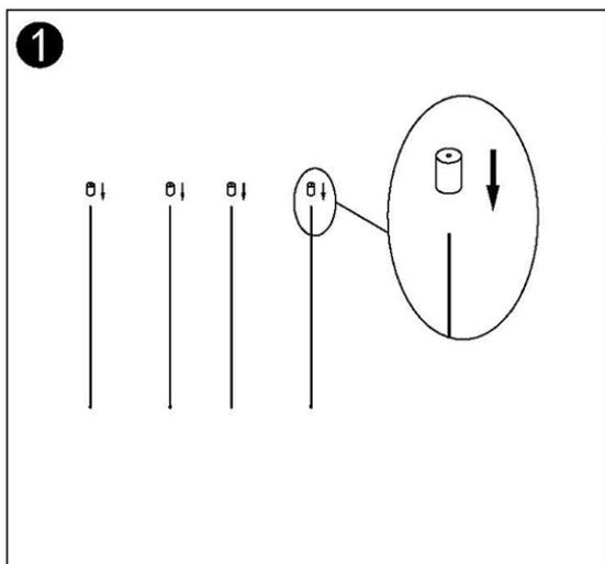
Thread the suspension wire through the wider end of the threaded collars and pull the wire all the way through the small hole until the “stop” is reached at the far end of each wire.
